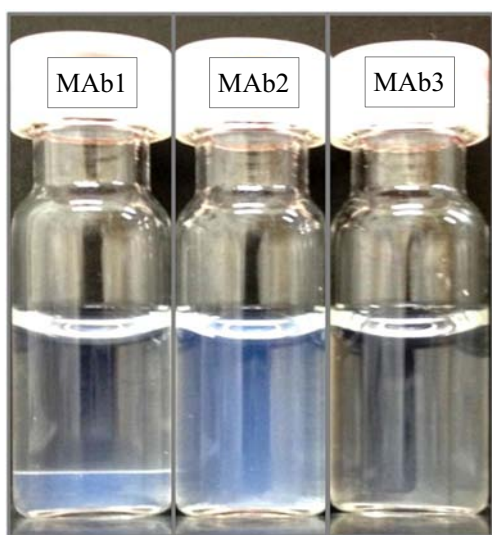
Fig. 5 Phase behavior of MAb solutions at a concentration of 60 mg/mL in 5 mM citrate/10 mM NaCl/NaOH buffer observed after 1 week storage at 25°C.
